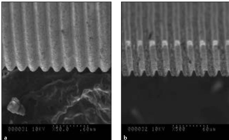
**Fig 4a** This SEM image shows the particle-blasted microthreaded region of an Astra Tech implant at  $\times 50$  magnification.
